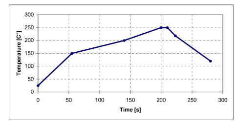
**Tolerance for Temperature settings T +0°C** (according to JEDEC J-STD-020C, July 2004) Used Solder: Omnix O338 (Sn95.5%/Ag4%/Cu0.5%), Alpha Metals Loetsysteme GmbH
